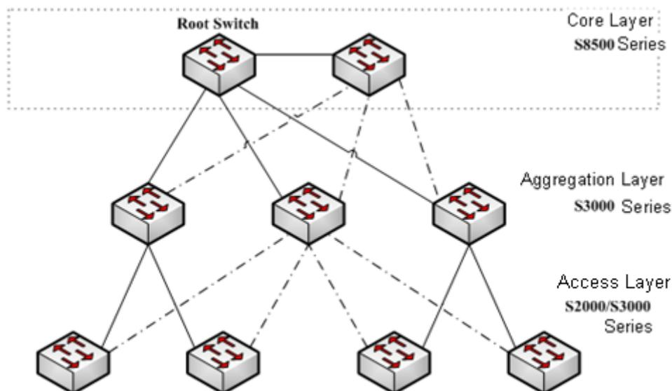
Figure 1.2 switching network topology
